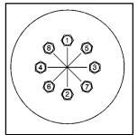
11. Tighten the nuts firmly in a crisscross sequence as shown by turning the ratchet clockwise, with the UP mark facing you.
